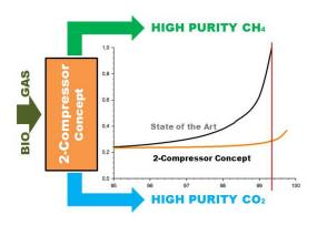
Fig1 Energy consumption (y) & methane recovery (x) of the 2-Compressor-Concept compared to state of the art technology
