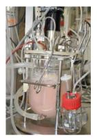
Culture of halophiles in a corrosion resistant bioreactor
