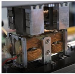
that stabilize variable loads in desired positions. An automated adaptation of the generated offset force, enables dynamic changes of the load mass and position, while maintaining a static power consumption of zero.
