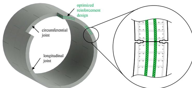
Left: Segmental tunnel lining structure.
